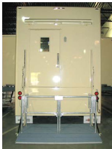
Lift Lowered with Handrails
