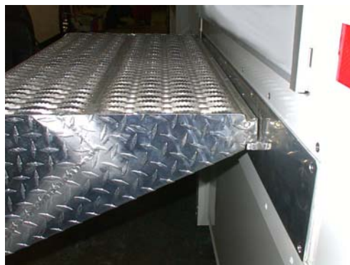
Figure 20: Stair Assembly (standard)
