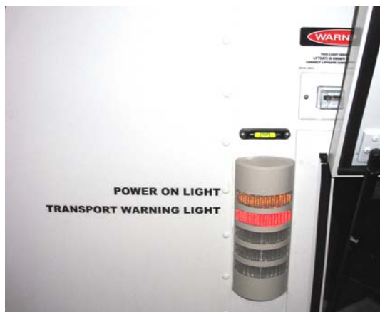
AC Power Light and Platform lift Transport Warning Light Figure 63: Warning Lights
