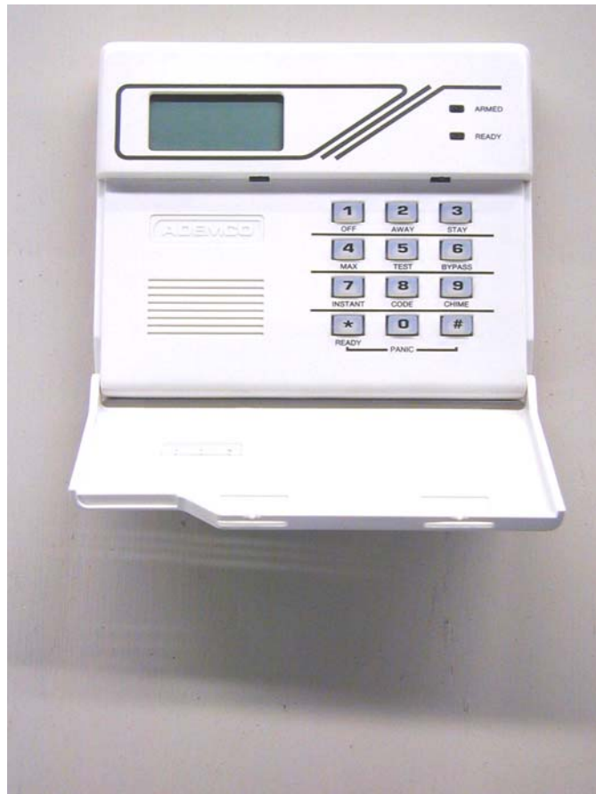
Figure 34: Intrusion Alarm Keypad
