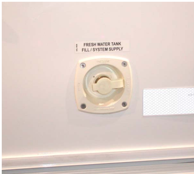
Figure 24: Fresh Water Tank Fill
