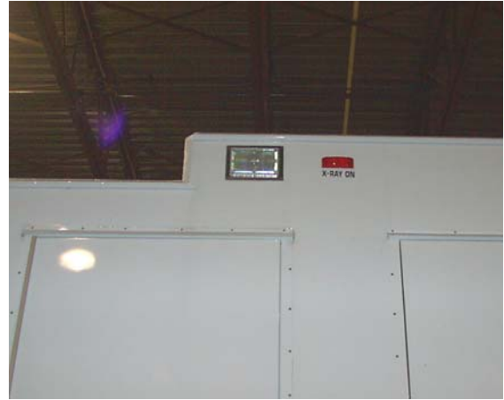
Figure 39: Entry Door Lighting
